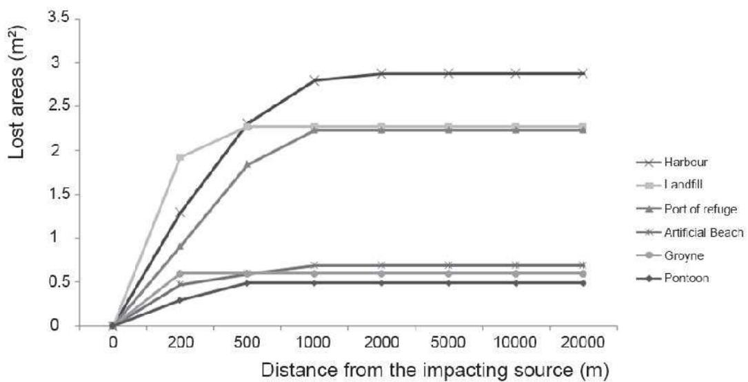
Figure 6. Lost *Posidonia oceanica* areas (in m<sup>2</sup>) according to the distance to different types of man-made coastline developments (96 facilities precisely) in meters. Results are presented for 1 m<sup>2</sup> of each type of development.
