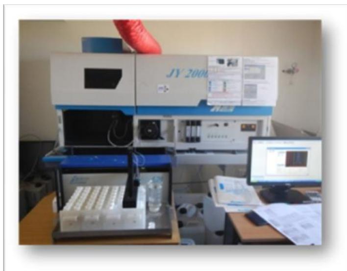
Figure 4.2-6 : ICP-AES Horiba-Jobin Yvon JY2000 Ultrace.
