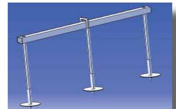
Model 4 : Sand screws with a coupling bar
