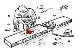
**STEP 6:** A final hit with the sledgehammer is required to drive in the remaining concrete rod.
