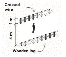
**3.** The third management phase consists in replacing the crossed wires with a single supporting wire.
