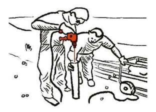
**Step 3:** With the wood bit, drill a hole in the centre of the post to a depth of 20 cm
