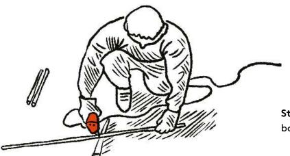
**Step 1:** Cut the reinforcing bar to a length of 40 cm
