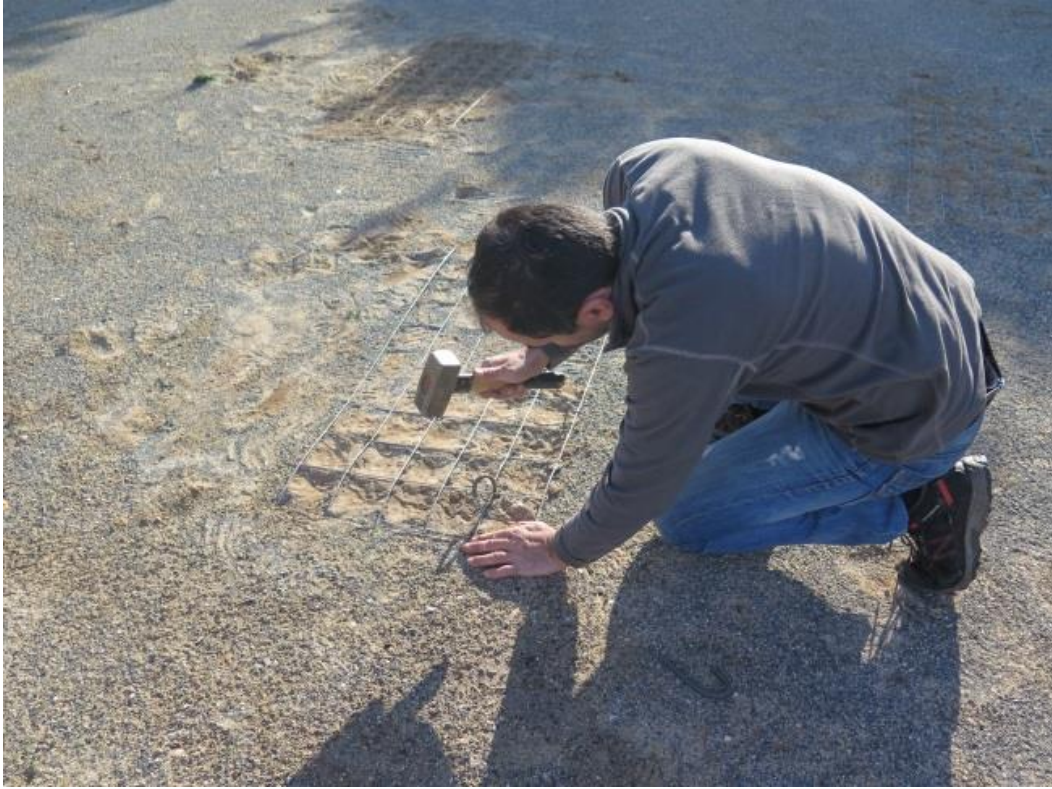
Photo 10. Example of a metal grid fixed to the ground
