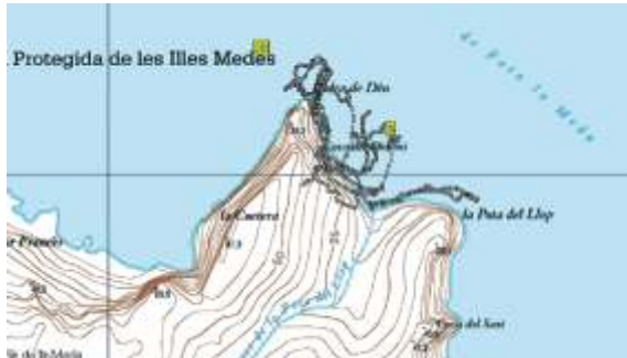
Orthophotomap interpretation in topographic format. What may seem to be GPS reading mistakes are due to the interpretations of cliffs. (Cartographic source from the I.C.C. - Catalan Cartographic Institute)
