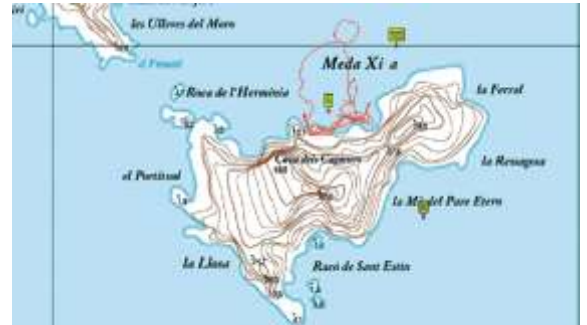
Orthophotomap interpretation in topographic format. What may seem to be GPS reading mistakes are due to the interpretations of cliffs. (Cartographic source from the I.C.C. - Catalan Cartographic Institute)
